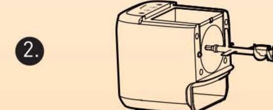
Insert the mixing paddle and secure it properly.
