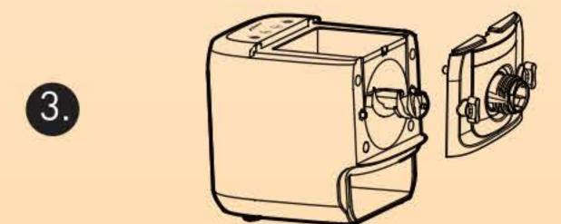
Attach the front panel with the mixing container/chamber unit.
