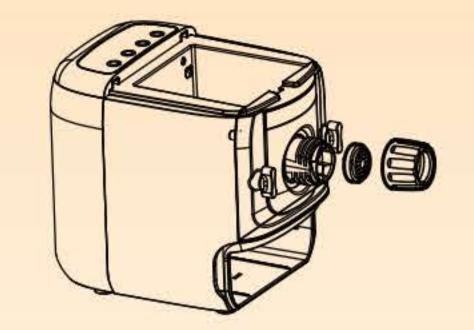
Install the shaping dies in the front panel. Before installing the shaping dies, wet it with a mix of water and edible oil.
