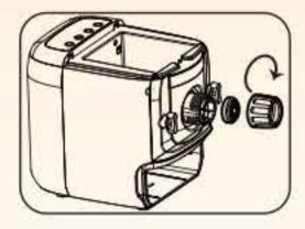
Remove the front panel by loosening the locking screws.
