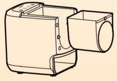
Place the mixing container/chamber into the appliance.
