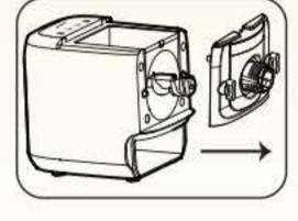
Remove the mixing paddle, followed by the mixing chamber/container.
