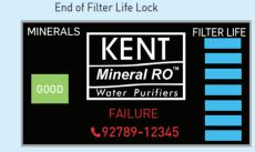
Service call number will be continuous ON. Filter Life all bars will be blinking If Product is in standby mode then Buzzer will Turn ON continuous Call service engineer for help
