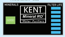
If the TDS level in the purified water is within the permissible range, the indicator would be in green Zone i.e Good
