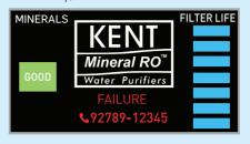
Failure and Call Service Icon will be 0N  $\,$  Continuously. UV Fault:
