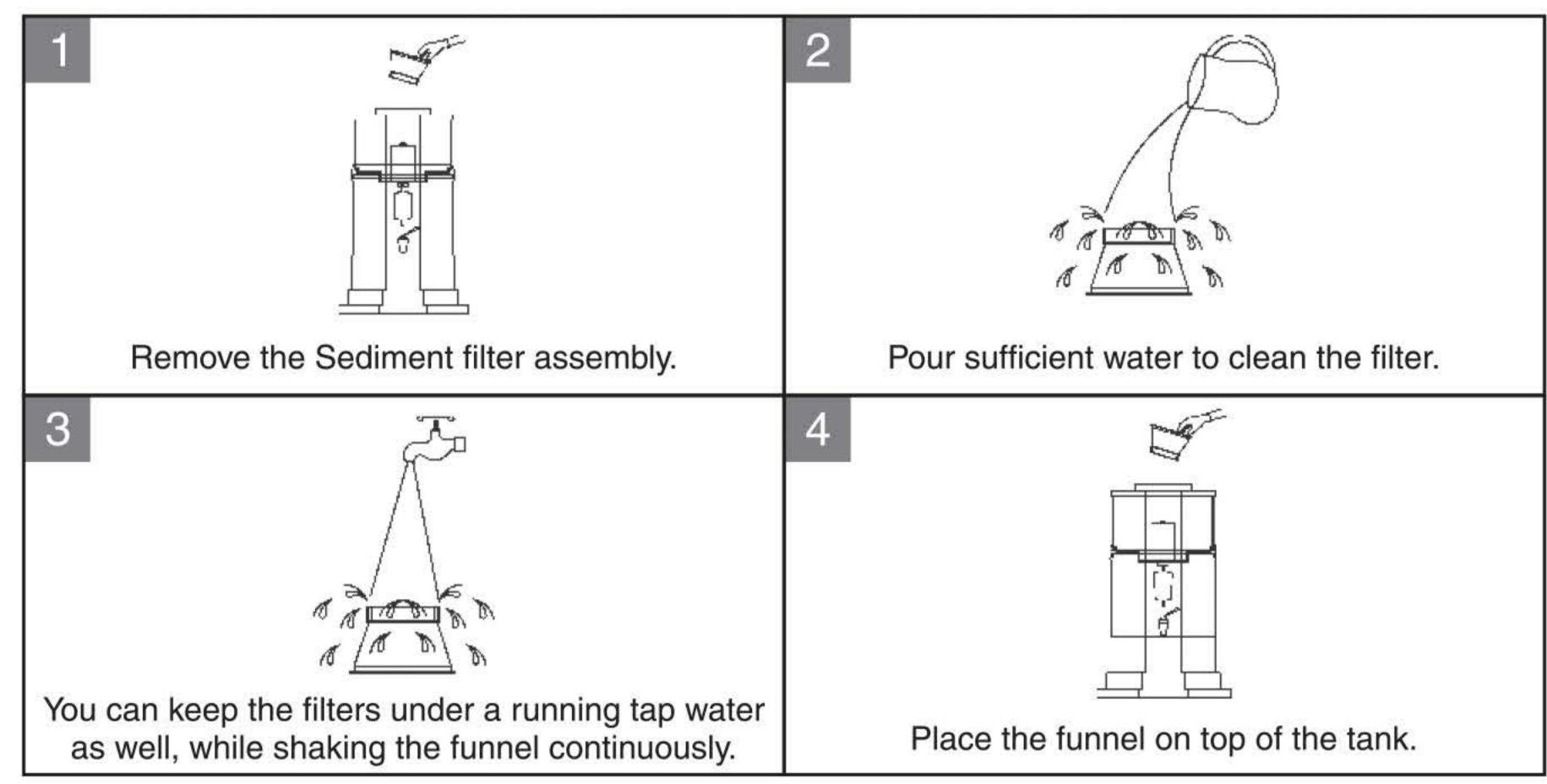
Frequency: The Sediment Filter should be changed after every 3 months.
