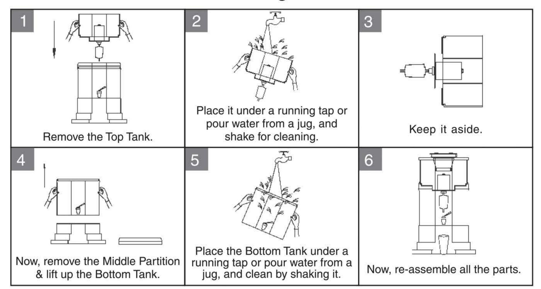
Frequency: Both water tanks must be cleaned once a week.
