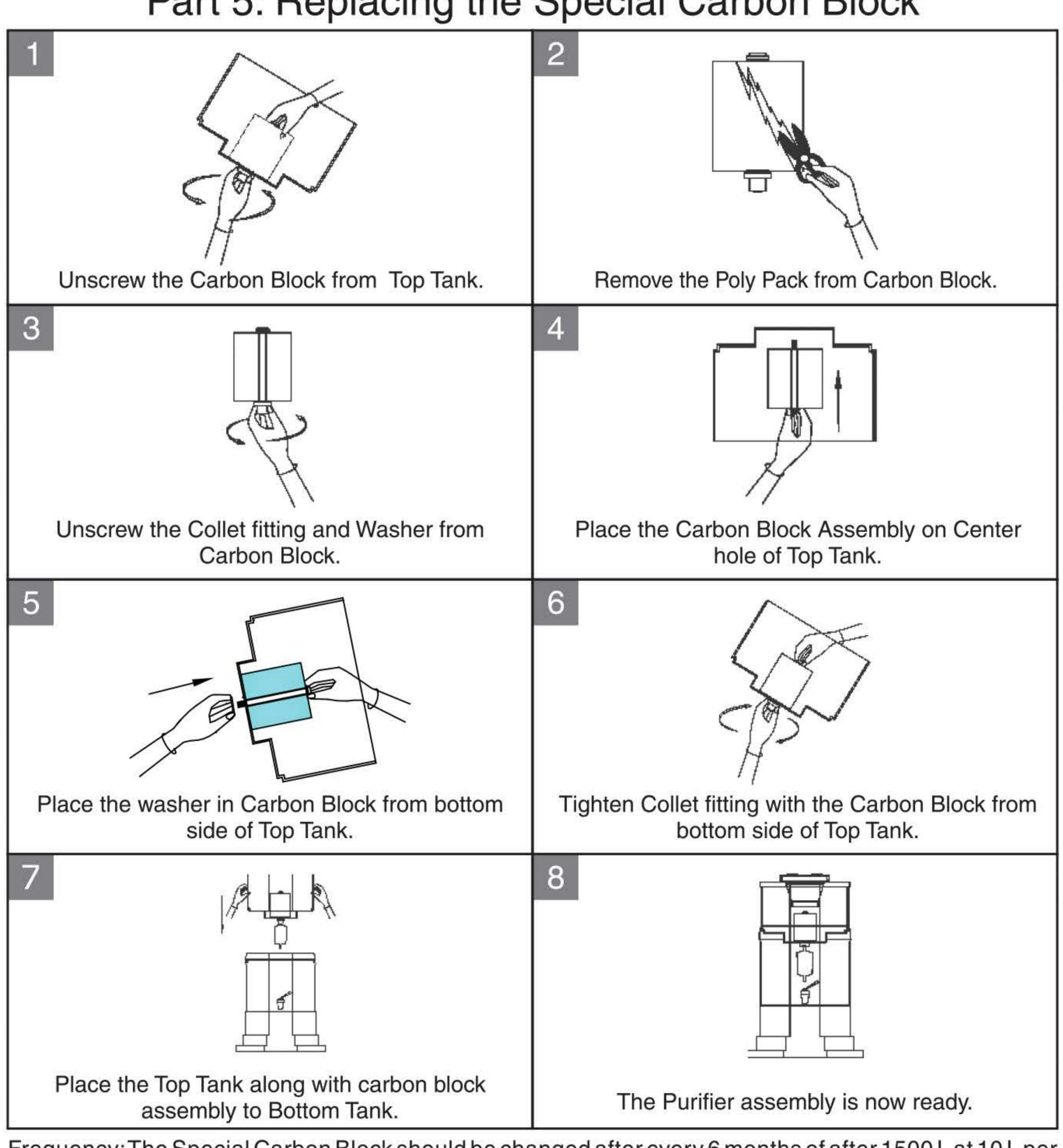
Frequency: The Special Carbon Block should be changed after every 6 months of after 1500 L at 10 L per day.
