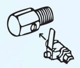
Attach threaded end of 3-way connector to raw water supply and plug-off the other end or connect to a tap.
