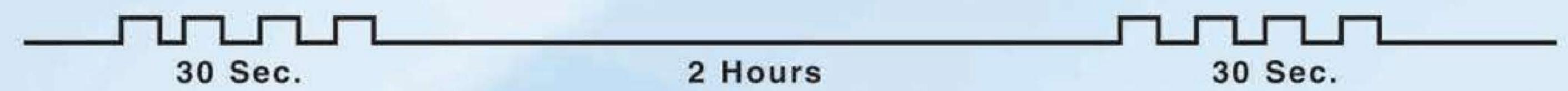
In case such an alarm is audible, please call the service technician and request him to change the filters of the purifier. However, if the filters are not changed within the next 60 hours of operation, the purifier will stop functioning to ensure purity and hygiene. The following alarm will be audible after 60 Hrs.
