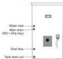
12. Connect the 3/8" White pipe to both the outlets labeled as 'Drain' for water drainage Water Inlet.
