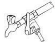
3. Connect the 3-way connector to the raw water supply as shown in the figure. The threaded end of the 3-way connector is fitted in line with the raw water supply. The other end can be connected to a tap or can be plugged off if not required.
