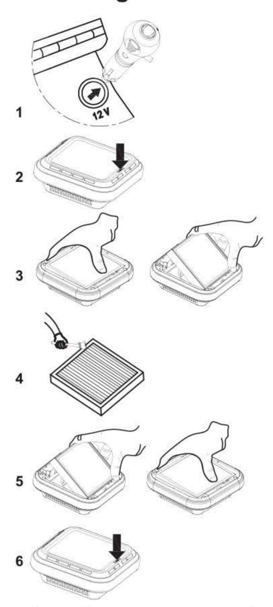
To ensure high efficiency, it is recommended to clean the filter cartridge on regular basis.
